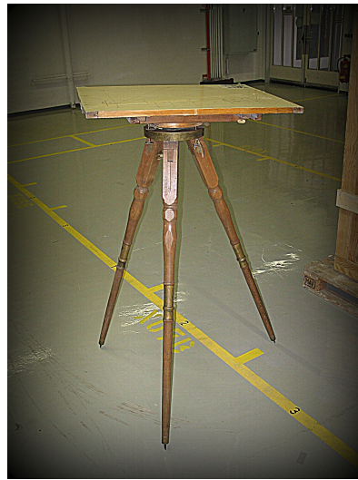
Figure 6: Original surveyor's plane table from Marinoni, Lombard, about 1770 (Vienna Technical Museum). Most probably the officers were equipped with a pattern of this type.
