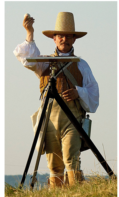
Figure 9: The author acting as surveyor at African temperatures with a light plane table. A billiard ball is used to adjust the table to the horizon.
